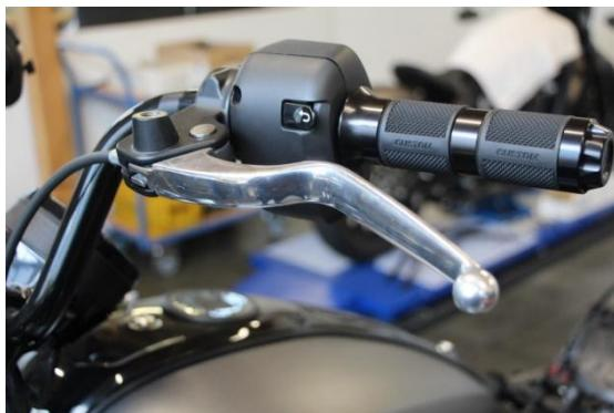
Completely remove the original lever.
