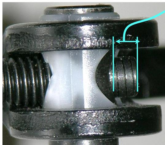
Carefully measure the protrusion at the thrust pin using a calliper and enter the measure below.
