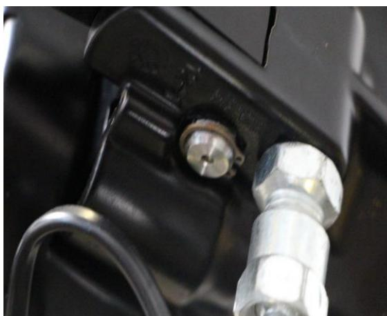
Remove the circlip or locknut of the bolt.
