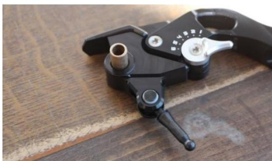
Remove the bushing from the original lever and push into the adapter with grease.
