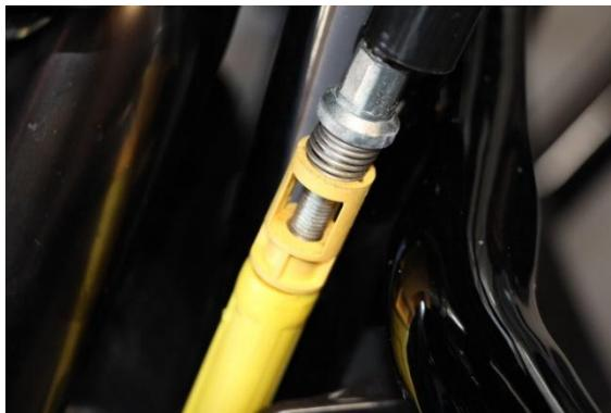
*Note: To remove the clutch lever the clearance of the lever might be increased with the set screw or the adjuster.*
