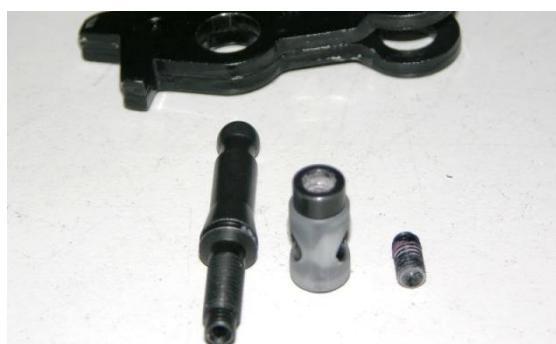
Unscrew the push rod from the guide pin and remove both parts from the original adapter.
