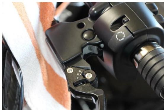
Mount the lever to the housing using the original the bolt (on the clutch lever mount the cable first).
