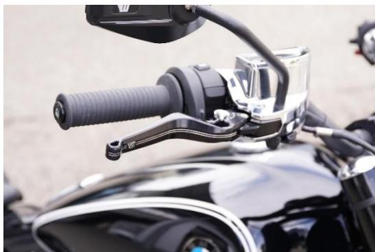
Next, mount the lever with the original screw and nut.
